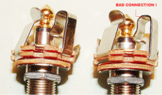
Check the tip and ring are making the correct contacts.
